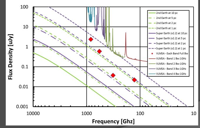
Direct Detection of 2<sup>nd</sup> Earth at 2 pc and Super Earth at 4 pc within 24 hr observations
