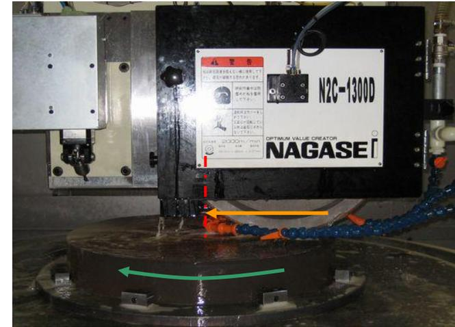
First Grinding P-V=0.7  $\mu\text{m}$
